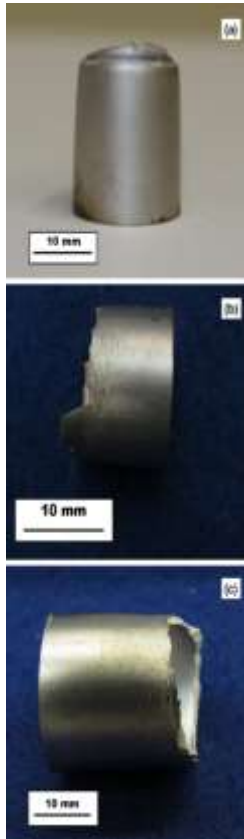
Figure 4 - Lateral view of as-received tensile specimen rupture: (a) H-free condition; (b) H-charged condition; (c) H-charged under stress condition
